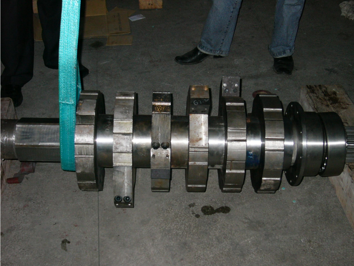
Stacking of the cutters and spacers on the main cutter shaft.
