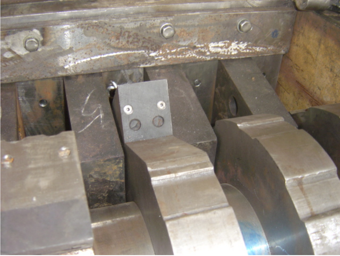
This is another view of the spacers and their top retaining bar which has been used on the Saturn and SSI designs for years.
