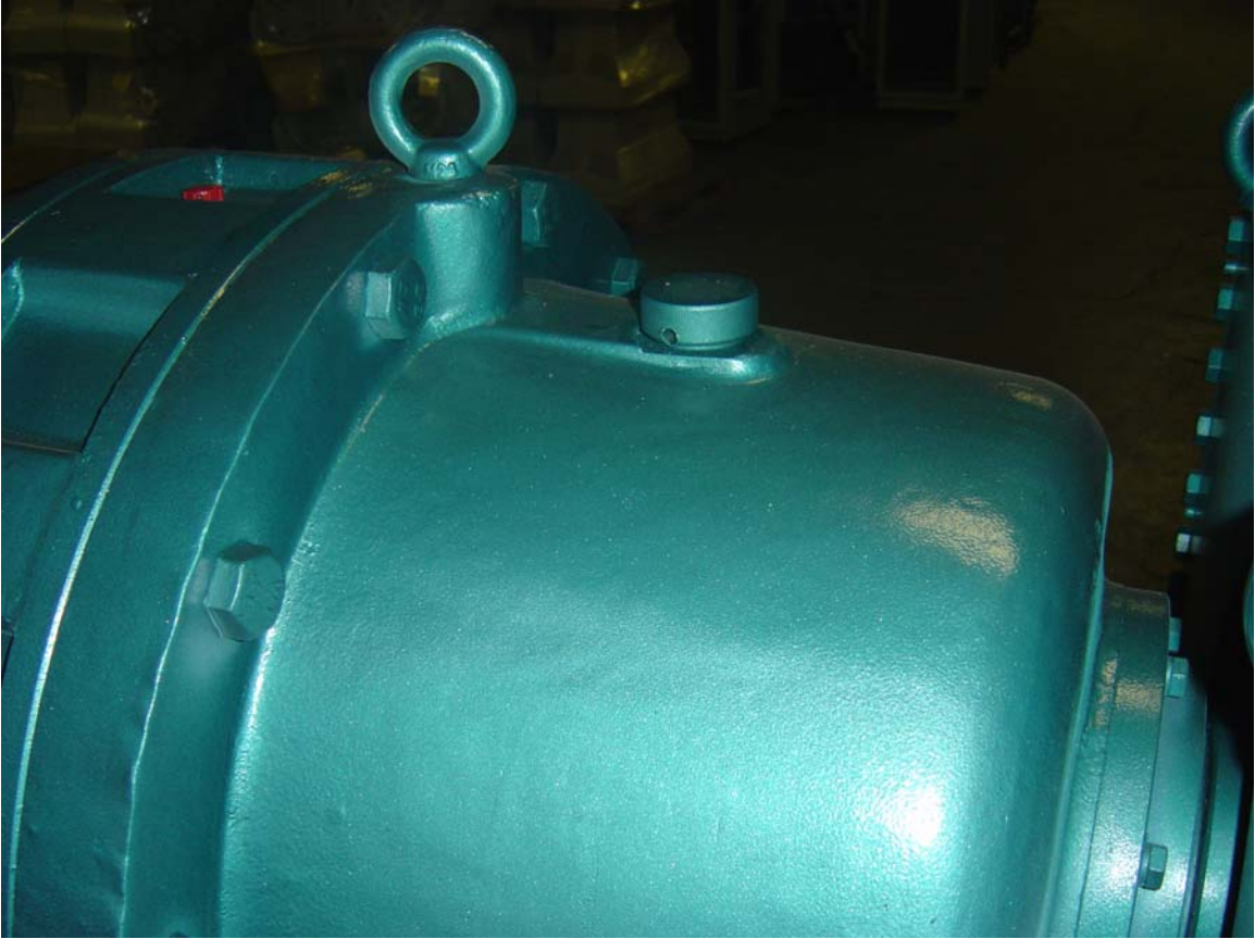
This is one of two Oil Fill Air Breather Cap found on most gearboxes.
