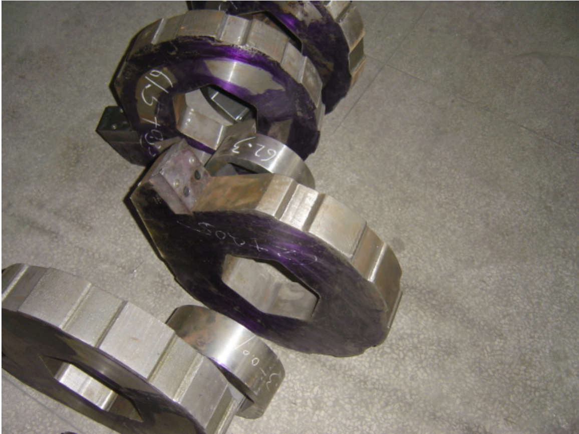
This is a view of the cutters that have a single hook and a ribbed outside for grabbing and a hex shaft design. These are for the Model 3434 unit and in this photo are about 2.5" thick and about 17" in diameter. Also seen is the spacer between the cutters.
